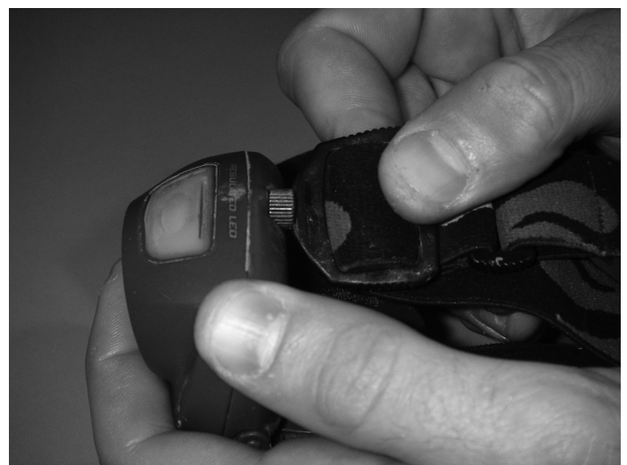
The screw for the battery compartment can be unscrewed by using the adjustment clip for the headband on the Quad. Photo by K. M. Kissell.
